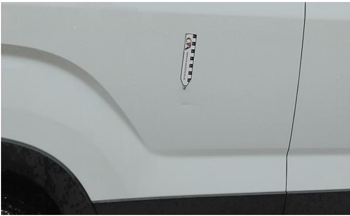
9: Door nsr Dented With Paint Damage
