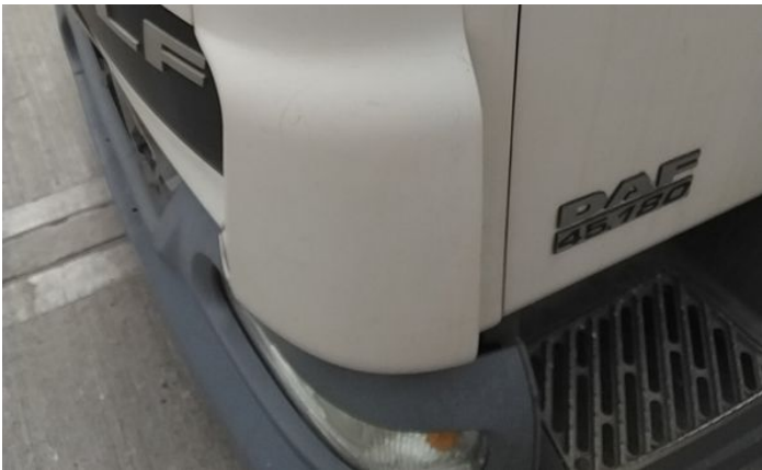
3: Bumper Front Grill Missing Replace
