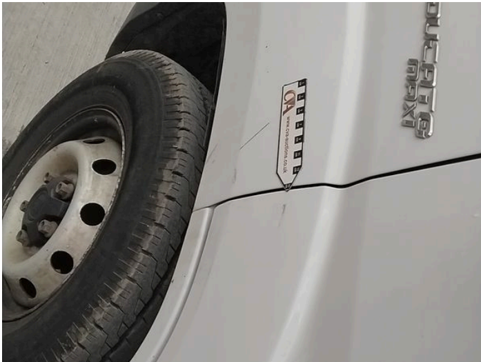
5: Door nsf Scratched Over 25mm Thru Paint
