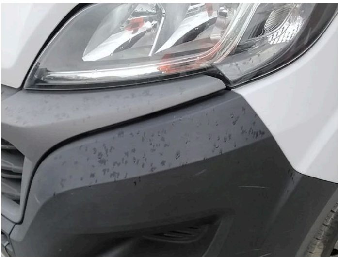
3: Bumper Front Moulding Scuffed (Unpainted) UpTo 100mm
