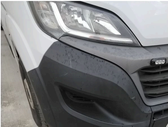
1: Bumper Front Moulding Scuffed (Unpainted) Over 100mm
