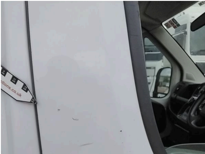
8: Door osf Scratched Over 25mm Thru Paint
