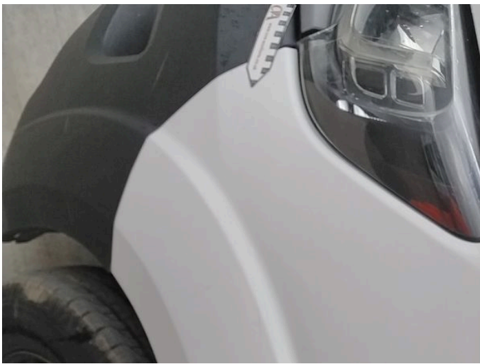
4: Wing nsf Scratched Over 25mm Not Thru Paint
