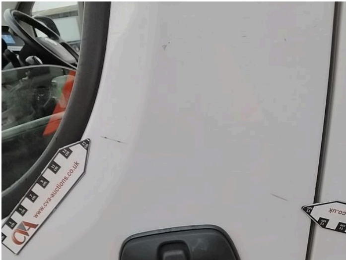
6: Door nsf Scratched Over 25mm Thru Paint
