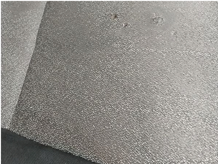
11: Seat Base Cover osf Burn Over 3mm
