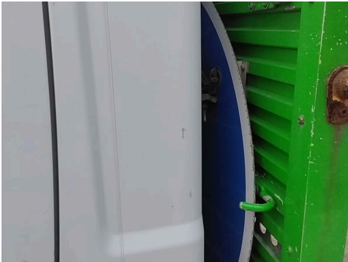
7: B Post ns Chipped Multiple Chips
